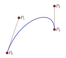
The curve begins at  $P_0$  and ends at  $P_3$ . The relationship between  $P_1$  and  $P_0$  defines the initial velocity, and the relationship between  $P_2$  and  $P_3$  defines the final velocity. In fact, we may write the Bezier curve as
