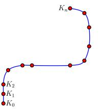
We created a Java program that allows us to move the waypoints and see the resulting trajectory. This allows us to easily design trajectories to accomplish various autonomous actions. Once the trajectory has been determined, we save the waypoints in a .csv file.
